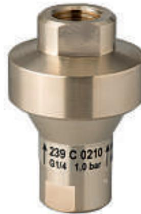
The EcoReg® fluid regulator is an independent diaphragm pressure regulator that can be installed in all fluid systems. The pressure regulator ensures a constant and precise output pressure independent from the input pressure. The pressure value has been factory preset and cannot be changed. This ensures that no one can manipulate the specified pressure value.
